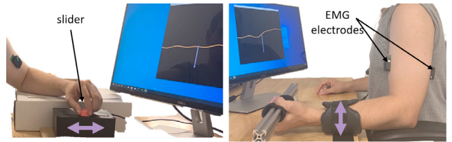
Fig. 1. Participants controlled a purple cursor on a computer screen using either a manual slider (left) or muscle EMG (right) interface. Adapted from Yamagami et al. (2020).
